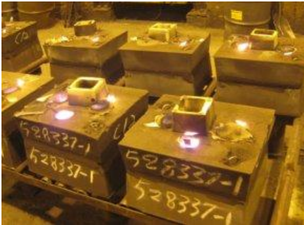
Figure 4: Filled sand casting molds.
