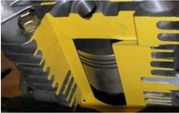
Figure 5: Cut-away view of piston and cylinder
